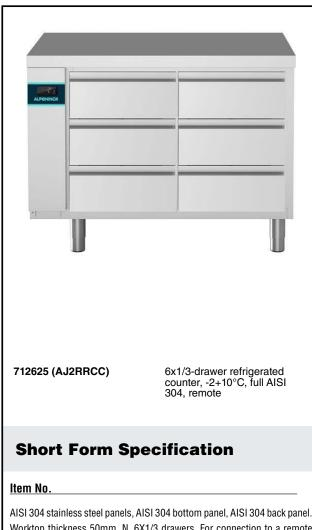
Worktop thickness 50mm. N. 6X1/3 drawers. For connection to a remote refrigeration unit (not included). Operating temperature: -2+10°C. R134a gas in refrigeration circuit.
